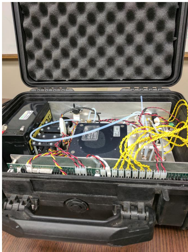
Figure 3. Engineering prototype of metal oxide nano-sensor integrated system with pre-concentrator
