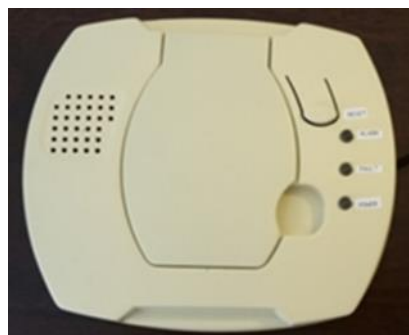
Figure 2: Package of MR Methane Sensor for UL Testing
