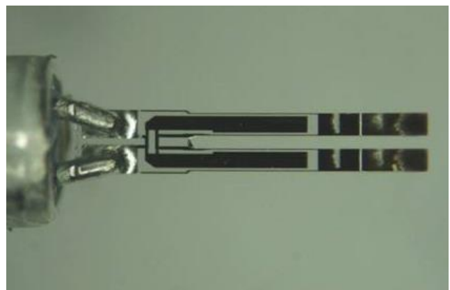
Figure 1: Tuning Fork Used in the MR Methane Sensor
