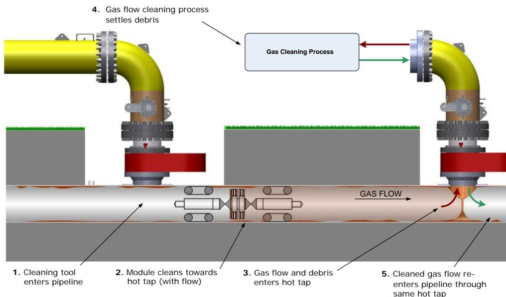
Figure 7: Cleaning Tool Configuration for full operation
