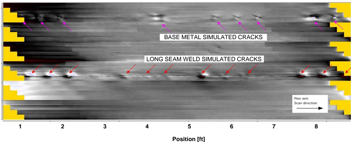
Figure 10: Crack test data
