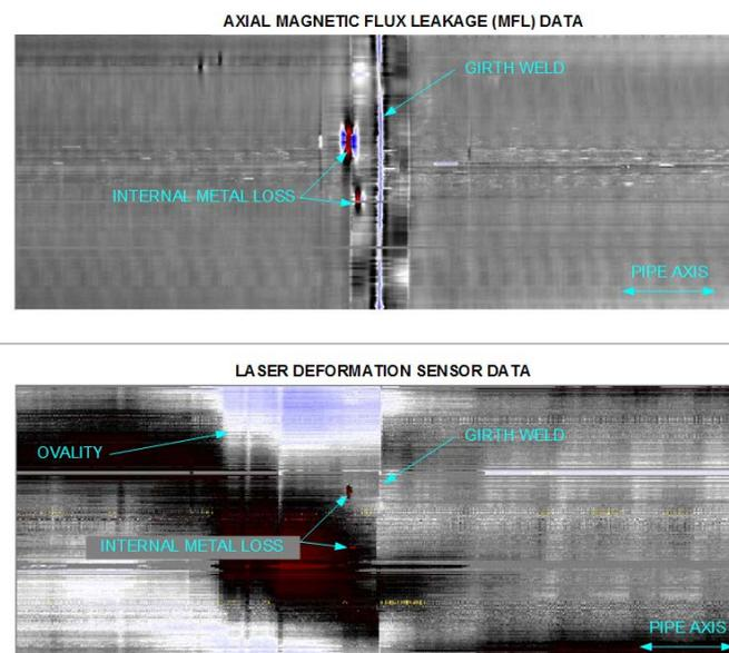
Figure 8: LDS Data from a Live Pipeline
