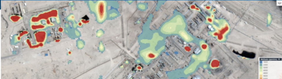
Image: Satellite image capture of detected methane leak emission plumes mapped over buildings
