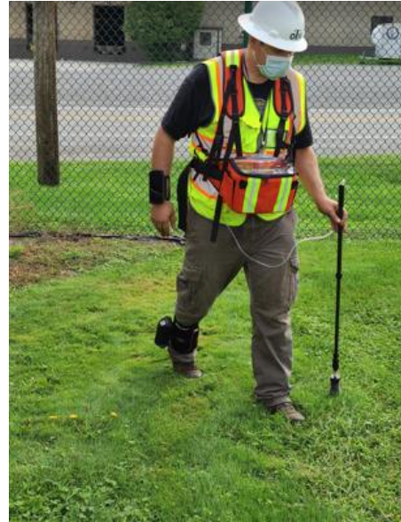
Figure 3: Leak survey testing
