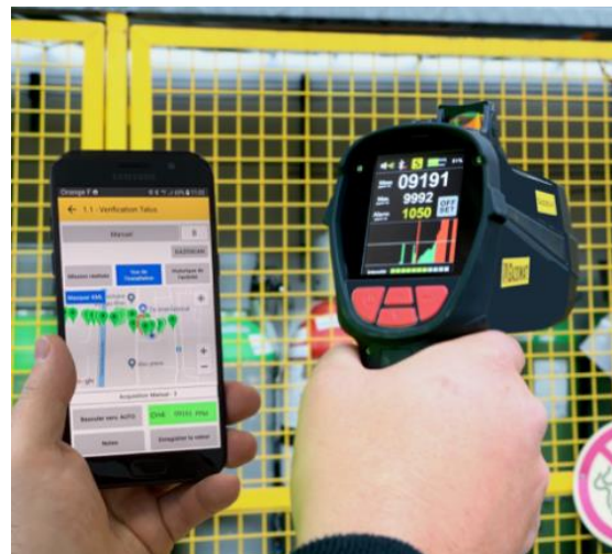
Figure 1: RMLD type methane detector with GPS tracking of walking survey and leak location identification superimposed on a street map and gas pipe map
