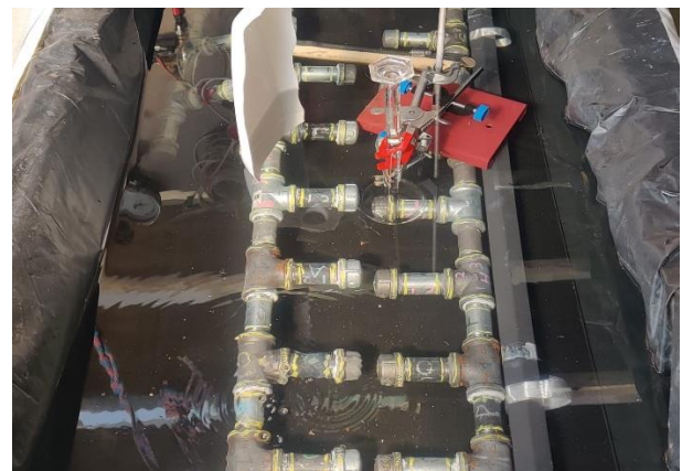
Figure 1 Experimental Set-up for evaluating threaded connections
