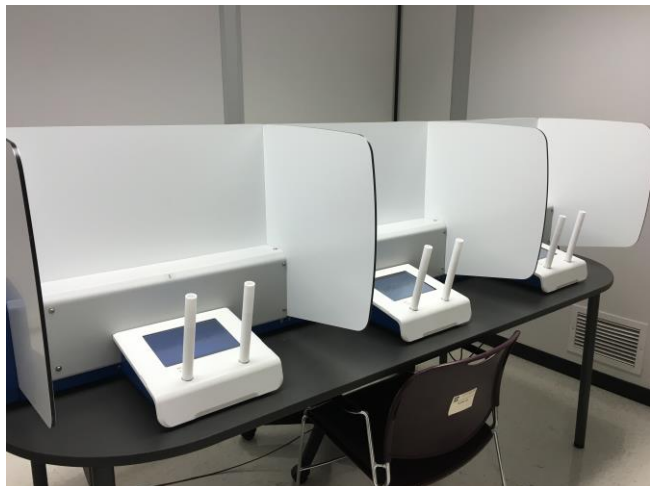
Figure 2: 6-person Olfactometer Test Setup
