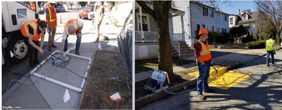
Figure 3. Setup and measurement using Surface Expression Method
